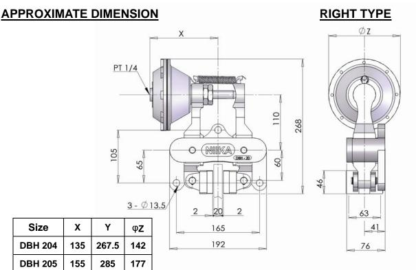
Warning: The initial torque on new units can be 30% to 50% less then the catalogue value until the friction facing and friction disc are lapped or worn in.
